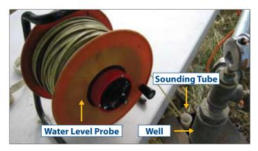
**FIGURE 5** Water level measurement using water level probe and sounding tube.
