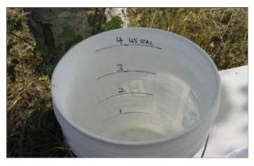
**FIGURE 4** A five gallon bucket and a stop watch can be used to estimate low pumping rates.
