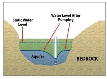
**FIGURE 8** Drawdown behaviour in small unconsolidated unconfined aquifer bounded by bedrock.
